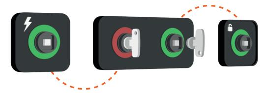
Power is isolated. The key can be removed and taken to the key exchange.
