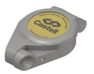
The Castell protective cap is used to help prevent dust ingress into the lock portion. The cap can easily be fitted to existing Castell locks. In addition, the cap can be also padlocked closed to prevent lock operation during maintenance.
