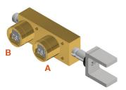
The switch cannot be switched on until key A and B are replaced in the KLC claw interlock and the claw is retracted.
