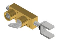
The KLC dual key claw interlock is a multi-key operated mechanical bolt interlock suitable for the control of electrical switchgear. The standard unit comes with a 16mm diameter bolt fitted with a claw that is used to control the rotation or movement of operating handles or toggles of electrical switchgear. The lock is manufactured in brass or stainless steel.
