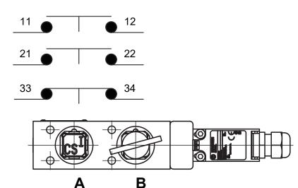
Primary Key (A) is Trapped & Secondary Key (B) is Free - Bolt is Extended:
