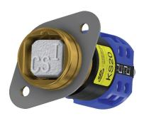
The KS is a key driven electrical switch designed for machine control circuits. This type of isolator should be used for short term, off load isolation. The KS lock is manufactured from either brass or stainless steel. The unit is able to be mounted into an existing panel or for surface mounting within its own polycarbonate IP65 rated enclosure.
