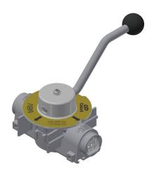
The Castell MBV modular ball valve interlock is designed to enable locking off, in either the open, closed or both open and closed conditions. The MBV is suitable for any quarter-turn valves including Ball, Plug and Butterfly Valves up to 3" bore size. Fitting the MBV enforces a logical, predetermined and safe sequence of operation where the control of flow paths is critical. The MBV is manufactured in stainless steel with stainless steel lock portions.
