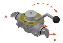
By inserting and turning key A in the MBV, the valve can be released from locked open condition and changed to closed. By turning and releasing the key B the valve is locked in the closed condition.
