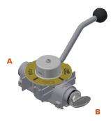
The service line is normally open and the MBV modular ball valve interlock locks the valve in the open position. Key A is free, while key B is trapped. Insert and turn key A to unlock the valve. Turn the valve to closed position. Turn and release key B to lock the valve in the new position.
