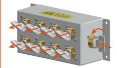
By inserting and turning the free end key in the Y key exchange box, you can release the trapped front keys in any order. Once the first key has been removed, the end key stays trapped. The released keys can be used in the access door locks to gain access to the hazardous area.
