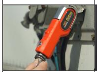
Step 9 Insert the key into the gladhand and turn the key clockwise to remove the gladhand from the coupling.
