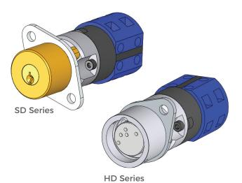
The KIRK Type PPS Power Panel Switch is a key actuated, rotary, two-position switch designed for isolation or switching of control circuitry. The Type PPS can be panel mounted or surface mounted with optional enclosure. It is available in switch ratings of 20, 25, 40, or 63A. The switch is UL listed and CSA approved.
