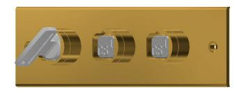
The B key exchange box is designed to enable the sequential release of keys (maximum 5) by the insertion of one or more initial key(s). The need for this type of product usually arises when there are multiple access points to the hazardous area. The unit will generally act as the link between the isolation locks and the access products. The product is supplied on a slim enclosure suitable for surface or panel mounting, and is available in different configurations of locks.
