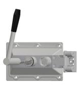
Under normal operating conditions, the isolation key is free, the personnel key is trapped, the catch is retained and the door is locked closed. Insert and turn isolation key, then release personnel key and release catch from locking mechanism by operating the handle.
