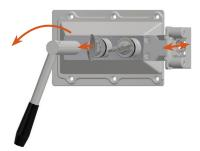
The door can only be opened when the isolation key has been inserted and turned and the personnel key removed. Once the personnel key has been removed, the handle can be operated and the door opened.
