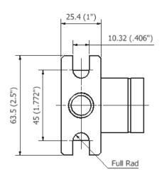
Mounting Holes: M8 (Brass) Ø8,35 (Stainless steel) Ø10,3 (US - Brass/Stainless Steel)
