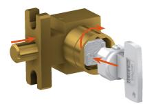
By inserting and turning the key in the bolt interlock, you can retract the bolt, e. g., releasing the disconnector. This will trap the key into the lock. Key is trapped, bolt is retracted
