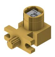
The KF Lock is a key operated mechanical bolt interlock for the control of electrical switchgear. The standard unit comes with a 16 mm diameter bolt of variable length, that is used to control the rotation or movement of operating handles or toggles of electrical switchgear. This lock is manufactured in brass or stainless steel.
