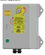
Turn the key to OFF position to switch the power off. A movement sensor in the MSI unit gives a signal to the solenoid once zero movement has been detected. This will illuminate a green LED. The key can now be released by pushing the green button. This key can be taken to unlock the access lock on the motor unit.
